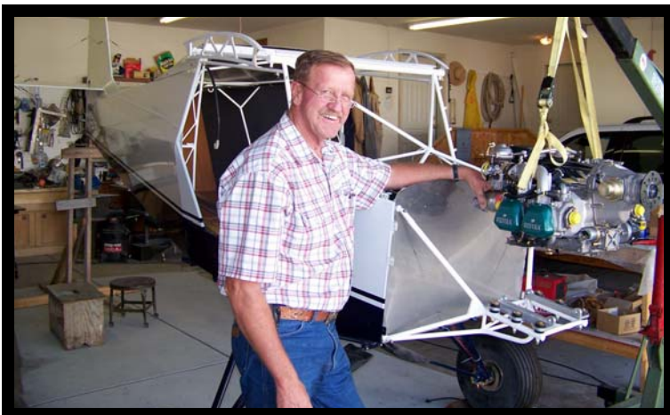
Roger Stout is almost ready to begin bolting his Rotax engine to his recently painted Highlander.
