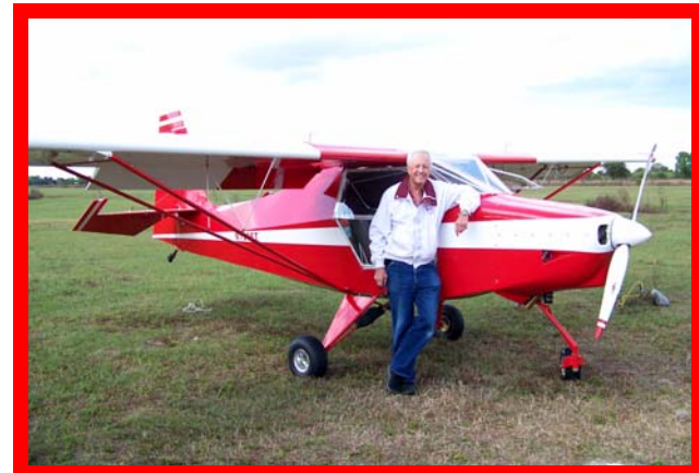
The nose wheel conversion makes the plane look quite a bit smaller, but it is much easier to land.
