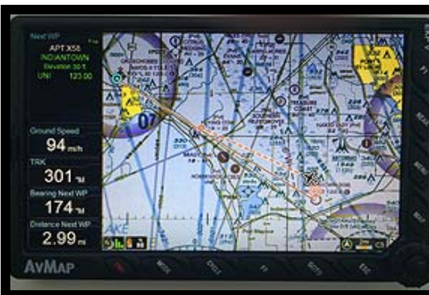
AvMap - Moving GPS map showing where I am, where I am going, how fast & when I will get there
