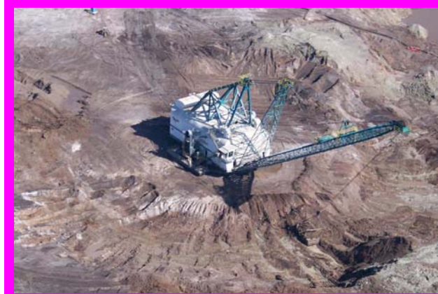
House sized drag line cranes work these mines
