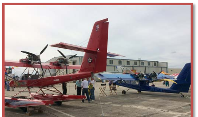
The AirCam looks like a twin engine open air flying canoe, & can be mounted on either floats or wheels
