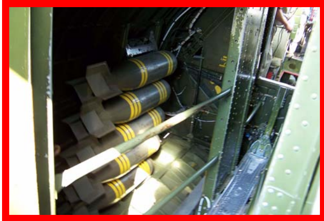
The Bomb rack for a total of 20, 500 pound bombs
