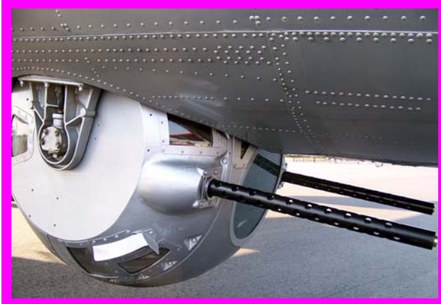
You had to be very small to access the ball turret (from outside only) The ball turret from inside the aircraft
