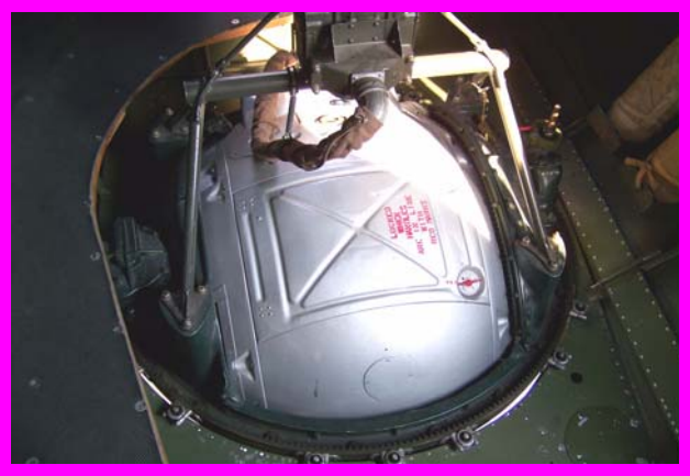
You had to be very small to access the ball turret (from outside only) The ball turret from inside the aircraft
